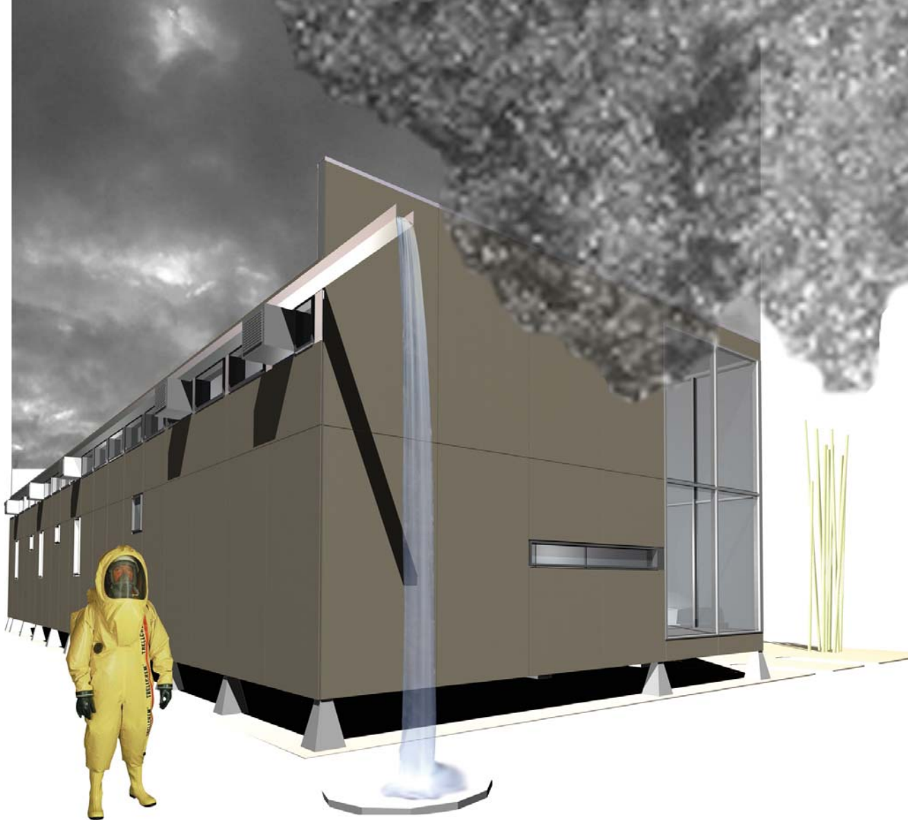
VIEW OF SCUPPER AND CISTERN
